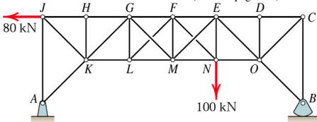
(5) Using the method of sections, determine the forces in members *CD*, *CJ* and *DJ*. (Meriam page 185)
