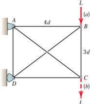
(3) The tower for a transmission line is modeled by the truss shown. The crossed members in the center sections of the truss are cables. For the loads of 1.8kN applied in the vertical plane, compute the forces induced in members AB, DB and CD.
